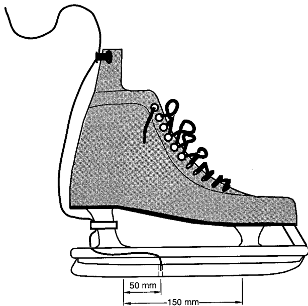
Fig. 1. Instrumented skate showing the flat bottom and thermocouple wire. The thermocouple wire enters a small hole in the side of the blade and connects to the thermocouple which is at the bottom of the blade.
